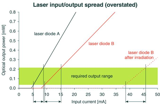
Figure 3: Exaggerated sample spread of the input/output characteristics of the laser diodes. The shaded area indicates the optimum light output power range, which can be reached by individual bias and gain settings in the Linear Laser Driver (LLD).
