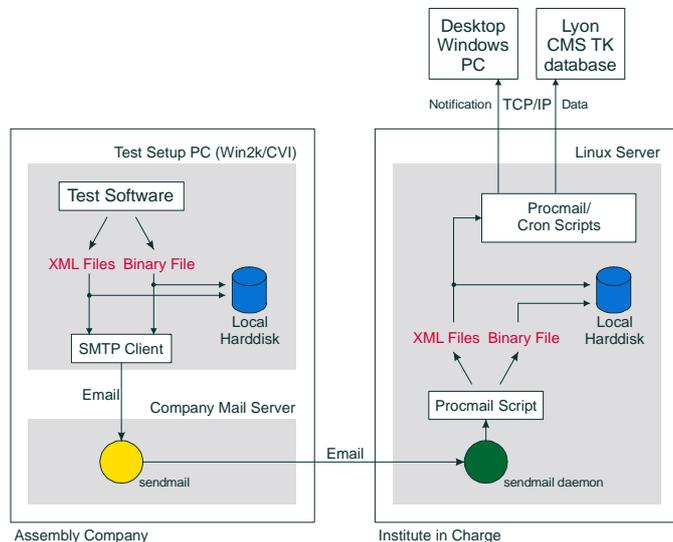
Figure 6: Data flow of the Analog Optohybrid (AOH) test results from the Automated Test Setup in industry (top left) through the company mail server (bottom left) to the institute in charge (right). Finally, data are submitted to the central database and a notification to a desktop PC is generated (top right).
