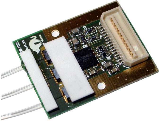
Figure 2: Analog Optohybrid (AOH) used in the CMS Tracker. The PCB dimensions are  $30 \times 23 \text{ mm}^2$  with the Linear Laser Driver (LLD) ASIC centered. The ceramic cover on top of the three pigtailed laser diodes protects the bond wires, and a similar piece is used for the fiber strain relief.
